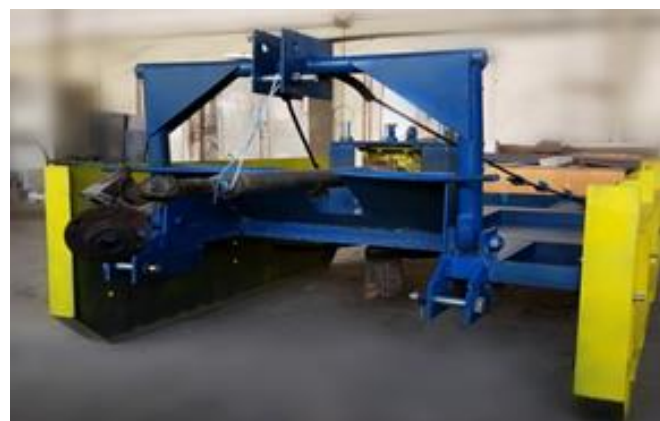
Fig. . 2. Machine for cutting and chopping bushes
