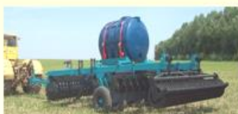
Disk chisel harrow БДВП-4,2-03 with chemical applicator
