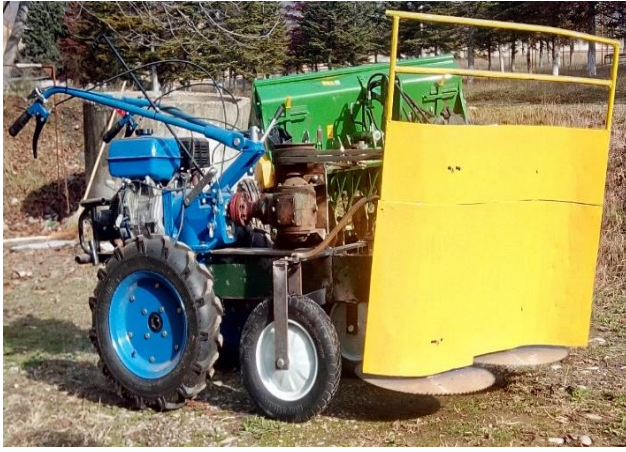
Fig. 3. Tea bush heavy trimming engine block aggregate.
