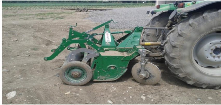
Fig. 2. Combined aggregate for soil loosening and arrangement of seedbeds
