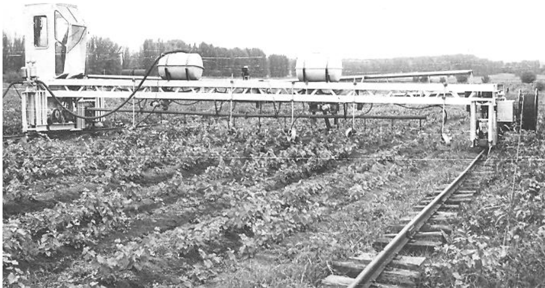
Fig. 1. Operation of the electrified bridge unit in the Kanda vineyard nursery.
