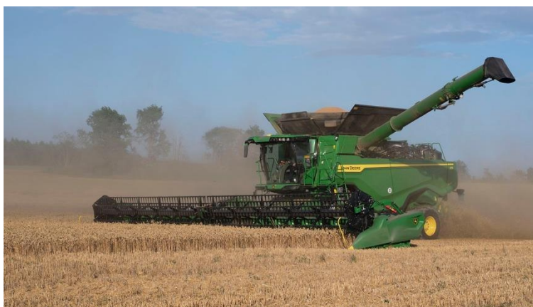
Fig. 1. This X9 combine from John Deere can harvest 100 tonnes per hour. Photo: Per Frankelius.
