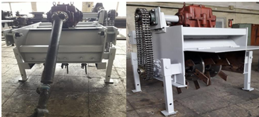
Fig.4. Mill-cultivator for uprooting the root system of plants.
