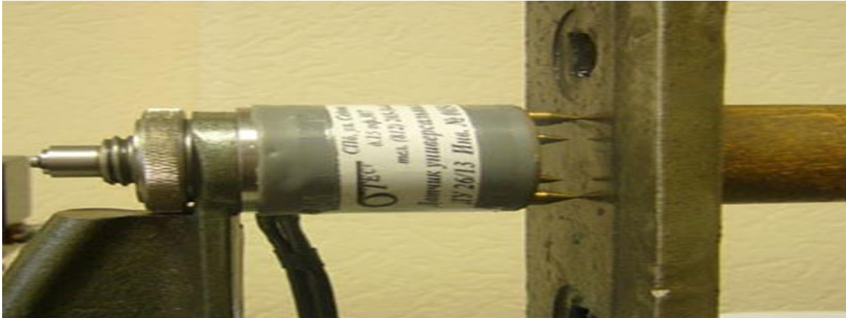
Fig. 2. Electrocontact sensor DU-26/13 fixed on the checked sample.
