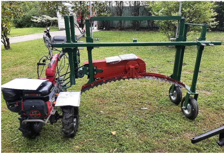
Fig. 1. Small-sized mechanized innovative technical tool for pruning tea bushes
