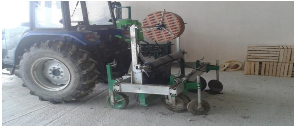
Fig. 3. The combined machine for laying of a drip system and plastic mulch
